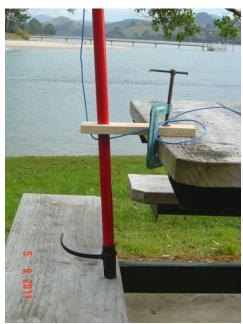
Method of clamping pole to table
