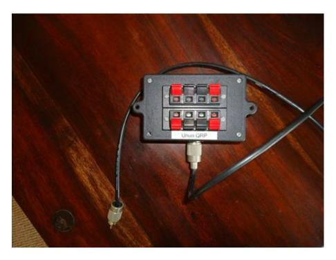
The counterpoises are just insulated wire cut to approximately a quarter wavelength on all the bands. The longest being 20 metres long for the 80 m band and the shortest being 2.5 metres long for the 10m band. I bound them together so that they don't get tangled up and soldered them all together at one point for inserting into the unun box. The counterpoises I lie along the ground in a straight line in such a way that they won't trip up any visitors.
