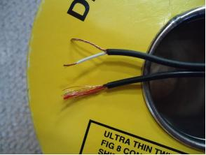
It is lightweight cable and very soft and subtle. The braid is not woven as in RG58 cable and is parallel with the insulated wire. It is perfect for wiring of keys paddles and speakers.
