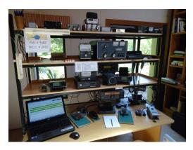
3rd shelf down. (L to R) A Galbraith paddle which is connected to my IC703+. Then a LDG M-1000 meter on top of a LDG AT-1000 Pro II Autotuner. A Kenwood speaker and above it an Icom IC-R75. Next comes the Icom 706 MKIIG with an Icom speaker on top.
