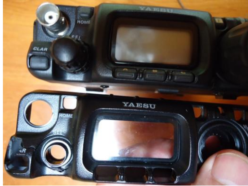
The bottom LHS of the picture shows the broken face.
