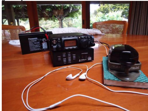
My set up for SKN. FT817, Czech Key and LDG Z-11 Proll tuner with Windom antenna.
