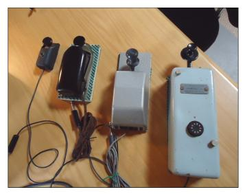
The picture above shows the difference in size of the four 4 keys. From left to right: Jardillier, Czech, Junker and Marconi.
