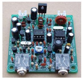
The Frog performed surprisingly well. Receive was crisp and clear, with a very nice sine wave side tone. Power output with 12v supply is close to 1.8 Watts as advertised. Now it was time to arrange a sked with Ian ZL2AIM. Ian using his K2 set at 5 watts with filter on, reported an RST of 559 a distance of approximately 150 km from my QTH.
